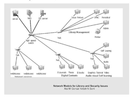
High speed library network model with three servers and one high speed layer-2 switch supporting four subnets The high-speed model as shown in figure-3 shows the server farm to switch connection is of 1000Mbps Gigabit t Ethernet.
